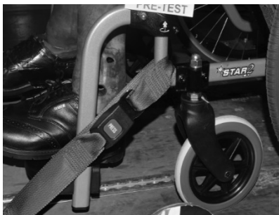
Fitting the front restraint
